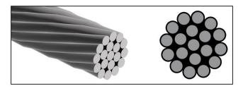
1x19 AISI316 stainless steel strand is a very poplar stainless steel construction. Used heavily throughout the marine industry, 1x19's excellent breaking load and low stretch characteristics along with its' aesthetic appeal make it a favourite for marine, structural and balustrade applications as well as many others, examples of which are shown below:
